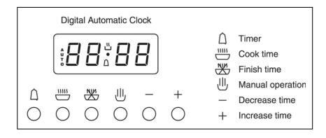
This appliance has a digital display 24 hour clock with six control buttons. When the power is connected, the screen displays 3 flashing numbers and **"AUTO"**.
