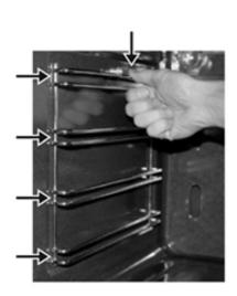
To remove the side support racks, push down on the wire below the locking pin and pull away from the oven wall until you can release the bottom of the support from the holes in the oven wall. To replace, reverse this procedure.
