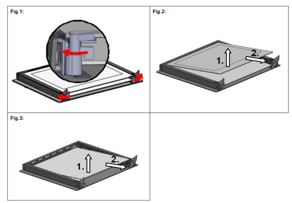
Reassemble the door by following the above procedures backwards.
